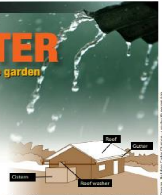
Figure 1. Above-ground rainwater collection and storage system.
